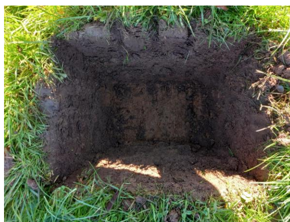
Photo 10: Test pit 1- topsoil 330 mm deep
